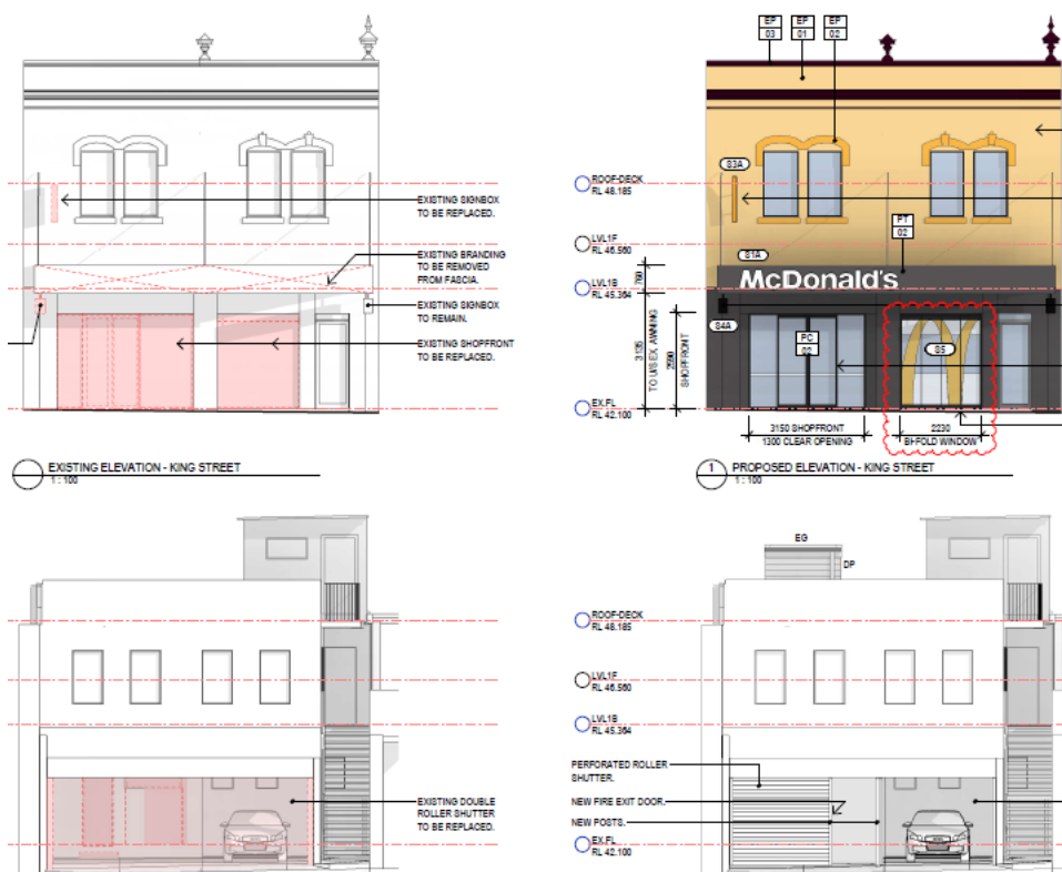
Figure 6: Existing and proposed front and rear elevations
